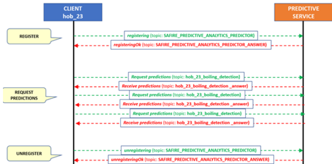
Figure 3-3 Client / PA Service interaction use-case diagram (Electrolux)
